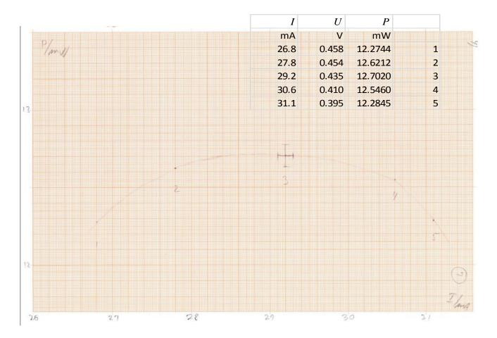
$$P_{\text{max}} = (12.7 \pm 0.1) \text{mW} \text{ at } I = (28.8 \pm 0.2) \text{mA}$$
